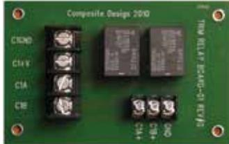
These Trim Relay Boards allow control of an aircraft's trim motors from the typical switches found in most stick grips. As the switches in the grips are too small to handle the motor loads and usually do not have the required number of poles, the 'TRB' offers a simple, elegant solution that is easy to wire and understand.
