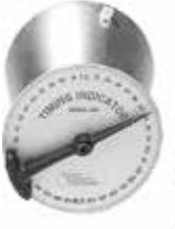
The Aircraft Timing Indicator Model E25 is a unique device that locates the relative relationships between the crankshaft, magneto point openings, camshaft and valve timing. Easily attached to the propeller spinner with mounting bands that are included with the unit, the E25 quickly and accurately (within 1/2 degree!) locates top dead center. The result: the all-aluminum Model E25 speeds up and improves the process of timing magnetos to the engine. With its easy-
