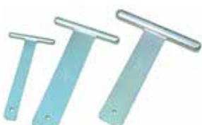
Simple, but necessary forming tool allows you to create new flanges or straighten out damaged flanges. Can be used effectively by taking to an existing body panel or locked in bench vise and create an exact radius edge using any flat faced panel beater or wood slapper. T-dollies are fabricated out of carbon steel hardened and zinc plated to provide years of service life. Extra long flat handle. Heads have radius ends.
