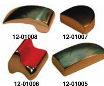
These professional series hand dollies are a complete selection of shapes and weights for most forming needs. These dollies can be used with panel beaters or wood slappers. Dollies weight and shape impacts the flow of the metal. Choose weights according to sheet metal thickness. Medium carbon steel, forged, ground, heat treated and mechanically polished for years of continuous use.
