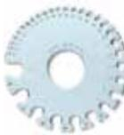
**#21 U.S. STANDARD SHEET METAL GAUGE** - The Sheet Metal Gage is for gauging uncoated sheet, plate iron and steel, based on weights in ounces per square foot. gauge numbers are in U.S. Standard. Numbers 0-36 (.325"-.007"). Made of hardened steel, with a satin finish for easy reading. Decimal equivalents on the back side. Measures 3-1/4" in diameter.
