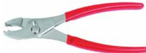
Specially designed for applying and removing spring hose clamps. The recesses in the jaws grip the ends of the spring so it cannot slip or twist. Grips with either end or side of jaws for reaching into tight places.
