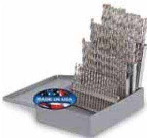
60 pc. Bright - Jobber Length - 118° Point - Wire Sizes - 95090850. Excellent general purpose drill bit. Precision CNC machined for faster, more efficient chip removal. Industrial-Grade NAS High Speed Steel (HSS). Heavy duty metal storage case. Numbered metal tip-out indexes keep bits organized. Made in the USA. Material applications: aluminum, copper, wood, plastic Size range: Wire #1-#60 P/N 12-04760 ..... **\$116.75**
