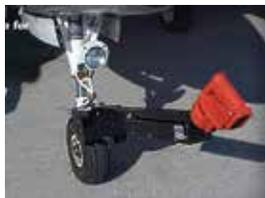
The all weather Robotow 24SL is lightweight (33 lbs.) and portable, making it ideal for carrying onboard your aircraft. When the Robotow's heavy duty all weather knurled drive drum is held against the nose wheel, the aircraft is easily moved. A trigger on the handle controls the speed while a switch reverses direction on command. Powerful, portable, and dependable, Robotow is an ideal power towbar for the aircraft listed.
