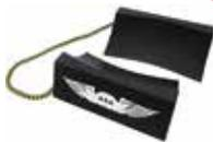
These tire stops are for keeping aircraft securely parked. A pair of black molded plastic wheel stops are connected with 22" bright yellow and black braided nylon rope that won't rot or retain water. The bottom cleats keep aircraft securely parked. Lightweight; 7-3/4" x 2-1/2" x 4-1/2"; concave design fits any aircraft tire. One pair is needed for each wheel.
