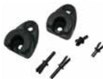
Many Piper aircraft have the same problem. The sun visor catches lose to stability, because the UV effect allows the plastic to become porous. These Piper Sunvisor Catches are made from a blended poly-plastic with a UV additive that will prevent UV corrosion. A set contains two pieces with the required plastic rivets. They are available in white and black
