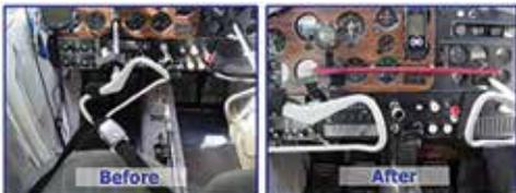
Rather than tying your seat belt to your controls, try AMC's new Airplane Control Lock. This lightweight control lock will stop your control surfaces from moving with the winds and will also prevent damage to your controls such as bending. This new Control Lock is lightweight and easily stored.
