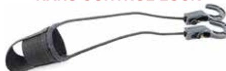
RANS has developed a control lock that attaches to most models. The lock consists of a bungee cord, a couple of hooks and cap that slips over the top of the control stick. Allows for bungee tension to be set for a particular model. Not hard bolted so if an outside force against the control surfaces occur, the bungees will absorb the load.
