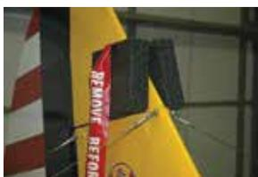
The Aileron & Rudder Soft Lock is made out of a durable foam that will not scratch your paint. Slides in gap between rudder and vertical stab. Keeps rudder from moving while plane is on the ground. Comes with "Remove Before Takeoff" flag. Patent Pending.
