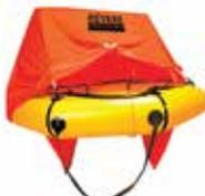
Double 200 lb. SuperRev™ ballast pockets, it enhances stability in rough sea conditions. Its light weight allows for easy deployment and the compact size makes stowage easy in the smallest of spaces. Operation is easy. Just open the red flap on the valise and extend the painterline. Give a hard pull and the raft inflates automatically in less than 30 seconds. Coastal Compact Raft is not recommended for offshore use.
