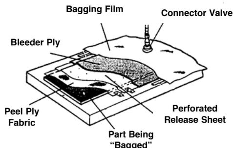
**VACUUM VALVE - TWO PIECE** - #8112 is a two-piece vacuum valve which requires one quarter turn to lock in place. Service temperature to 500° F. This valve is an industry standard The base is anodized and is red in color. Inside Diameter: 1/4" standard. Threads: 1/4" NPT. P/N 01-14855 .....\$29.85/ea.
