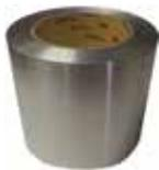
3M Interam Mat I-10A, 49 inches by 25 feet (one roll): Ceramic fiber based material that expands into low-density insulation blankets when exposed to high temperatures or flames. Outer foil layer is aluminum.
