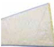
Ultra-light FAA compliant Thermal/Acoustic Insulation by the foot. The blanket consists of a covering film qualified to Boeing Material Spec. (BMS) BMS8-377 Ty I & II, Cl 1 and fiberglass qualified to BMS8-48 Ty III, Cl 2, Gr A.
