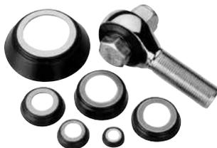
Protect the spherical bearing of rod ends. This patented design features a neoprene rubber seal bonded directly to an aircraft quality washer. The seal encapsulates the bearing and flexes accordingly with any change in angularity. This provides unprecedented protection from dirt and other types of contamination which may severely shorten the life of these important components.
