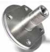
Includes mounting flange and backing plate. Mount your gascolator solidly on the firewall with this special bulkhead fitting. Simply drill a 5/8" hole through the firewall and a backing plate on the cabin side and rivet the 1-1/2" x 1/8" flange to the firewall. Connect the incoming fuel line to the AN6 male tube fitting on the cabin side. Screw the gascolator onto the 1/4" male pipe (on the engine side). Machined from mild steel (303 stainless steel) .....P/N 05-00907 .....\$21.85
