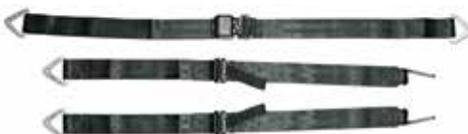
Specially designed for the VariEze, this popular combination is also used in the Long-EZ, Quickie, Q2, Cozy, Sea Hawk and several other homebuilts. The belts are made to fit snugly, and the aluminum end fittings save weight. Order two sets for all above aircraft except Quickie which uses one set. Not FAA approved for certificated aircraft. P/N 13-01300..\$539.00 Set
