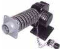
The Frosty dc motor is the same as our FAA PMA 6 port blower and has been STC approved as well. The blower's footprint is an ultra small size measuring (3.50L"x 3.50W"x 4.50H) for the blower, universal mounting bracket and speed control module. This ventilation kit is compatible with Experimental, Sport, GA, Rotor-craft, Business, Commercial aircraft, as well as Land-Mobile, Marine and Military Vehicles.
