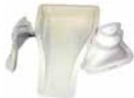
This large NACA scoop is the largest inlet available anywhere. 0° axes of air flow 17", 90° axes total width, 10 inches with a 9" x 2" outlet or 18 square inches. A separate two-part duct can be purchased separately. This allows the user to take the air directly into a 2" or 4" hose connection. High impact polycarbonate, formed at 375° F.
