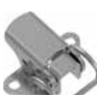
These Dzus over the center type latches are used extensively on cowl doors and other applications on aircraft such as Cessna, Piper, Grumman, and many homebuilts. Model II latch: This latch provides 220 lbs. of ultimate strength and 45 lbs. of working strength. Pull up ability is .2 inch. Mounting holes will accept .156
