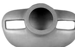
Originally made for the Thorp T-18, this cowl has been used on several other types. The starter ring is enclosed when used with the Lycoming. Makes a nice front end on the CA-61 & CA-65. Measures 35"W by 19.5" high. Face of center opening 13-1/2" O.D. P/N 05-01176 .....\$173.80
