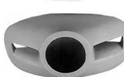
This nose cowl was designed for the T-18 pressure cowl system. A 4-inch prop extension is required and it is generally used with the MC-5 Bottom Cowl. Measures 36" wide by 20" high. Face of center opening 12-5/8" O.D. P/N 05-00551 .....\$180.75
