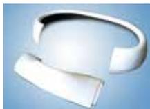
Styled after the Piper Comanche, this cowl can be used on just about any homebuilt powered by the Lycoming engine. It is made in two parts, allowing the easy removal of the cowl without having to remove the prop. Used on the following airplanes: Starduster I and II, Playboy, EAA Biplane, Jodel D-11, Tailwind, Tempete & the Skybolt. Measures 35" wide by 21" high. Will accommodate a spinner approx. 12" in dia. P/N 05-01180 .....\$172.75
