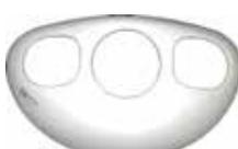
Same shape and size as used on the Piper PA-14. Can be used on the same aircraft as listed for the MC-3A design. For builders not wishing to use an electrical system and is seen on most Pitts Specials built for competitive aerobatics. 35" wide x 21" high. Center opening 9-1/4" dia .....P/N 05-01184 .....\$175.75
