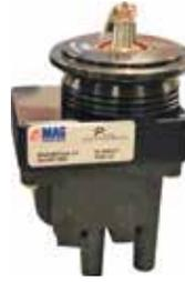
Of all the E-MAG innovations, the self-powering capability of the "P" Model is the most significant. It solves the largest single issue faced by all electronic ignitions - their need for an uninterrupted power supply. Power back-up strategies that a) compromise ignition effectiveness, b) solve only half the problem, or c) require additional maintenance are less than ideal. Next-Generation ignitions need a better solution. So what does a next-generation electrical back-up need to do?
