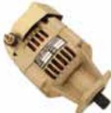
The BC410-H is the original high-performance spline-driven alternator that mounts on a standard vacuum pump accessory pad. It may be used either as a primary or a stand-by alternator for a nominal output of 20 to 30 amps, depending on engine RPM. Designed for many hours durable service, the BC410-H features a dynamically balanced rotor,
