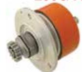
The 200G is a 12 amp 14V gear-drive alternator for Continental engines (C-75 through O-300). Features a ultra-reliable, brushless design, with a billet aluminum mounting flange and heavy-duty ball-bearings. Used in the prototype Vari-Eze, as well as many Cassuts, Q-200s, and other home-
