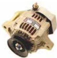
The L-40 is a high-performance belt-driven 40 amp alternator for Lycoming engines. Designed to meet the rigorous demands of weight-sensitive homebuilt designs, without sacrificing reliability, the L-40 alternator features a precision-balanced rotor, sealed heavy-duty ball-bearings and 2 internal cooling fans. Weighs 6.1 lbs. and measures 3.9" (diameter) x 5.6" (length). Also
