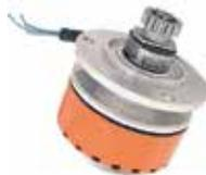
The BC433-H is a 30 amp 14V gear-drive alternator for Continental engines (C-75 through O-300). Featuring a unique brushless design, with a billet aluminum mounting flange and heavy-duty ball bearings, the BC433-H is an ideal choice for a
