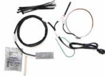
The Reiff preheat system for Rotax 912 and Rotax 914 aircraft engines is an engine-mounted electric preheat system designed for easier cold-weather starts. The preheat system consists of a 100-watt metal "hot strip" element, which is epoxied to the bottom of the crankcase, and a 50-watt band heater that is clamped to the oil tank.
