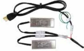
HotStrip is thin and lightweight like a silicone pad, but made of aluminum for maximum durability. Works either as a stand-alone sump heater or integrated with the Hot Band Cylinder Heating Systems in the Standard, Turbo, and Turbo XP Systems. Bonds to the bottom or side of oil sump and electrically heats the oil. Features dual heating elements for redundancy. System includes two 100W elements thermostat, and power cord.
