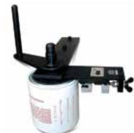
This tool was designed to eliminate much of the mess that occurs with small hand-held oil filter cutting tools. Very simple to operate, it is excellent for individual aircraft owners as well as FBO's and maintenance shops where a lot of filters need to be cut. Simply clamp in a vise, screw on the filter, turn the cutter into the filter and hand crank to open the filter. The rugged construction enables this tool to operate trouble free for years.
