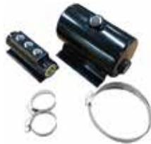
The Raven Full Oil System includes a CNC machined adjustable valve. There are no extra holes to plug, you simply rotate it to where you want it. The system includes the valve, mount and clamps, as well as the air/oil separator, mount and clamps. Both the valve and separator use stainless steel internal parts and are powder coated for durability. The weight of all components is 4 1/2 lbs.
