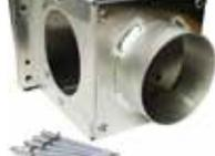
P/N DL-001 - This cabin heat box has been engineered to be the smoothest, most efficient and lightest heat box built. Fabricated from aircraft-grade aluminum with stainless steel shaft, arm and flapper. Originally designed for use on the popular RV-4 homebuilt, but is applicable to most other designs. Total weight is only 5.2 ounces.
