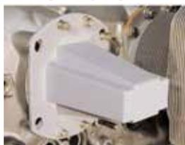
Install TopCap in place of a removed cylinder to protect the engine from dirt, debris, and stray parts. Made from fuel and solvent resistant polymer, TopCap allows for full crankshaft rotation. One size fits Lycoming wide deck 320, 360, 540, 720 and Continental 470, 520, and 550.
