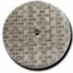
**Two Styles Available:** Cut & Polish/Unitized Wheel-7A Medium grade (harder) Use to radius and deburr edges of aluminum parts. These wheels give a uniform brushed satin finish to parts and deburr quicker and easier than hand finishing. These wheels are discs of Scotch-Brite web compressed and bonded to form a rugged, dense wheel. Wheel size: 6" dia. x 1" wide x 1/2" thru hole..... P/N 12-00875 .....\$99.75
