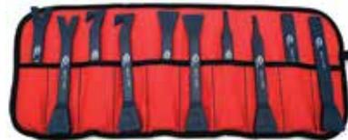
PolyScrapers are offered in a convenient Red Canvas Pouch with black trim. The kit contains 10 Polyscrapers, each having its own pocket. Pouch can be rolled and secured with black tie. The PolyScraper Kit comes with multiple tips for various sealant removal situations. There is a forked blade, a unique push/pull design, a wide blade, a .25” narrow blade, and a straight blade. ....P/N 09-02458 .....**\$82.75**
