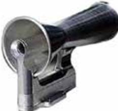
This venturi develops 4" Hg suction from double-throat venturi and 10" long horn. Used to operate a directional gyro or gyro horizon. When operating a directional gyro there is sufficient capacity to also operate a turn/bank. All aluminum construction. May require a suction regulator. Wt. 0.9 lb.
