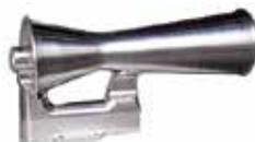
This "super venturi" is similar in appearance to the 4" venturi but with redesigned air passages and a recontoured, long (11-1/4") horn. It pulls enough vacuum to operate a gyro horizon, directional gyro and a turn/bank. Must be used with a suction regulator
