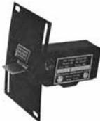
Warns by light and horn of any danger of an approaching stall regardless of the flight maneuver. Never signals unless a stall is imminent. Consists of an instrument panel unit (fits standard 2.25" hole) containing a warning horn & signal light, and a small vane wing unit which operates a relay. Operation of the instrument doesn't depend upon air speed but rather on the air flow conditions of the wing. Complete with installation kit & instructions. Installation time: 2-6 hours.
