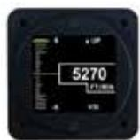
The VSI200 is the most accurate Vertical Speed Indicator available for your aircraft. It exceeds all the requirements of TSO C8e and AS8016A while providing the following functionality: • Installer selectable for 0-2,000fpm, 0-3,000fpm, 0-4,000fpm or 0-6,000fpm rates of change. • Graphic bar indication of rate of change • Precision digital rate of change indication. • Fits standard 2-1/4" mounting hole. • wt: 4.3 oz VSI .....P/N 10-006271 .....**\$758.00**
