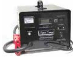
Designed to supply filtered DC bus power through standard APU receptacle in private and commercial aircraft. Up to 25 or 50 amp is available for operating avionics and flight control systems when the master switch is activated. It can also charge the battery through the plug at a 10 amp rate. Output is current limited, and will withstand starting loads. Voltage is limited to prevent battery overcharging. DC Current and voltage are displayed on panel meters, voltage accurate to 00.00
