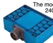
The model TC240 VDC/VDC Power Converter that supplies 240 watts of 5 to 18-volt power to electronic equipment, including lighting and cabin accessories.
