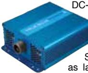
DC-to-AC static inverter produces 115 volts at 60 Hz for 500 watts of "wall outlet" power from an aircraft's 28 VDC input. Has the same connector and footprint of legacy designs, plus overload and short-circuit protection up to 150 percent of the rated load.
