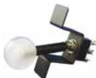
Canard and Non-Canard RED / GREEN lighted Retractable Handle with DPDT Lever Lock Gear Switch (12 VDC / 7.5 amp, or 24 VDC / 4 amp ) Gear DN the handle LED light is GREEN; Gear in Transit or is Unsafe, or the Canard Retractable Handle and Switch is in the Center OFF position, the LED light in the handle is RED; Gear UP the handle LED light is OFF, or BLUE (your choice).
