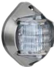
SunTail™ serves as an LED Anti-Collision Strobe and Position Light designed for the tail of the aircraft. SunTail™ can synchronize its strobe with any of AeroLEDs™ LED lighting products. SunTail™ does not require an external power supply and will retrofit the mounting footprint of legacy lighting. It is TSO-C30c Type III and TSO-C96a Class II approved. Available for 12V and 24V systems - No external power supply needed - Low power consumption - 5-year warranty
