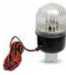
Measuring only 4" high by 2 3/4" diameter, it weighs less than 5 ounces! Special dual xenon flashtube arrangement provides ultra-bright flash visible for over 3000' in daylight, much more at dusk and dawn. No separate power pack is required, all electronics are fully contained in the strobe itself. Lens is available in clear, red or green. Each strobe draws less than 300ma.
