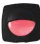
Recessed mount convenience light. 3 Bright LEDs behind a frosted panel. Recessed mount with hardware. Dimensions: 2.25" x 2.25" x .5" depth. #6 mounting holes with snap on cover. 12 Volt DC or 24 Volt DC, very low power drain (0.1mA). Applications: Mounts flush into foot wells, door panels, and side panels. Ideal as a convenience light, mp light, or chart light.
