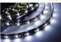
This flexible 15 ft LED Lighting strip is powered by 12volts, is adhesive backed and waterproof - allowing you to install it in any location you want light to glow. This LED Lighting strip can be powered directly with 12v as a light source for footwells, dome lighting, passenger areas, etc. LED Lighting comes in Red, White, and Blue with a black flexible PC Board technology, and clear silicone-based flexible covering..... P/N 11-14143 ..... \$19.75
