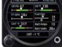
The GI 275 EIS variant can serve as a primary EIS display for piston engine, fuel, electrical and other data. Use dual GI 275 displays to monitor twin-engine aircraft. Graphical display of cylinder head and exhaust gas temperatures allows you to pinpoint the optimal fuel/air mixture for efficient power management.
