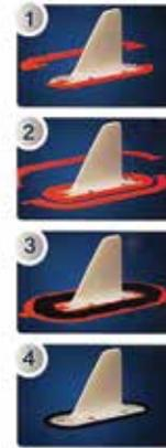
Custom designed templates improve the antenna sealing process, making it more precise, efficient and cost-effective.
