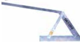
**MODEL 4** - Wing tip VOR antenna designed for smaller tips with a 10 degree flare on the top portion and a curled aft portion. VSWR less than 2.0:1 over the frequency band of 108 to 118Mhz.
