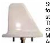
Streamlined Transponder Antenna. Non-TSO'd for Experimental aircraft. The Delta Pop Aviation streamlined transponder Antennas are the best non-TSO'd antennas we have found, and they offer a low drag solution at a good price. Frequency - 1030 to 1090 MHz. VSWR - Less than 1.2:1 Measured with Anritsu Antenna Analyzer. Polarization - Vertical. Impedance - 50 Ohms. Connector - BNC Female. Mounting - 8-32 x .437" long threaded studs. Weight - 2.6 oz / 74 grams. Finish - White Polyurethane.
