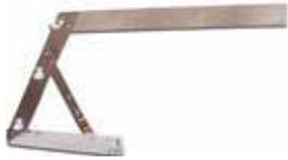
**MODEL 1A** - This Wing Tip Com Antenna is designed to fit inside larger fiberglass wing tips on metal (conductive that is) airplanes such as T-18's, RV's Bonanzas etc. But tuned out for the Com Band. The wing tips must have internal dimensions of at least 11"x24" and generally fit better
