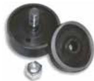
Reversible cutter for both 2-1/4" and 3-1/8" instrument panel holes. Easy to use even with instrument panel installed in aircraft. Allows for close work with other instruments already installed. 4 lbs (2Kg) shipping weight.
