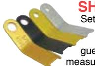
Set of four gauges for -3, -4, -5, & -6 rivets. Each gauge measures MINIMUM height and MINIMUM diameter of shop heads AFTER setting. Eliminates guessing if your rivets are properly set. Works for measuring both universal head and flush rivets. Precision machined to size from 2024 aluminum. Rivet size permanently stamped on each gauge. Color coded anodized finish. Instructions included.....P/N 12-00631 .....**\$22.95**
