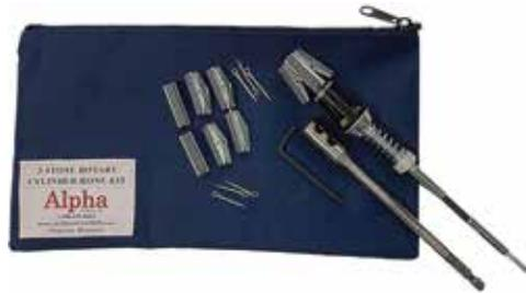
This 3 Stone Rotary Cylinder Kit makes available an effective tool to recondition the interior running surface of the oleo cylinder barrel, and is intended to be used each time the MLG oleo struts are disassembled for routine seal replacement or when upgrading to the popular Main Landing Gear Oleo Restoration Kit (STC SA01247CH).
