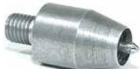
innovative paint cutters. They work by slicing through the paint around the head of the screw so you can remove it without chipping the paint. They have a 1/4x28 thread to fit into any angle drill or you can get the optional arbor (p/n 12-02460) for use in a drill chuck. Does not work on dome head rivets. 1 lbs (0.5Kg) shipping weight.
