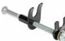
You know how hard it is to get at the springs on the push rod tubes... Now, you can compress them and remove the tube in under a minute. Just slip this tool onto the spring and crank the shaft counterclockwise (an air ratchet works great for this) to compress the spring, and then give everything a wiggle and out it comes. It's a must-have tool when working on big bore Continentals. This tool will fit all production engines Lycoming, Continental, Franklin, and even most old radials.
