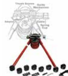
This portable, hand-operated roll type swaging machine will swage MS type terminals onto galvanized and stainless steel cables from 1/16" diameter up to and including 3/16" diameter. Includes machine, a full set of roll dies, terminal gauges and feed guide adapters & instructions in a steel carrying case. Wt. 95 lbs. New manufacture. All replacement parts available. Special order.
