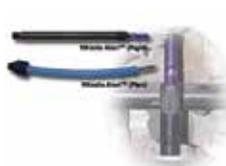
No more burning your fingers and hands! Just Listen! Insert Whistle Alert™ into any 14mm spark plug hole and bump the engine until you hear the whistle. You are now on the compression stroke! • Easily find Top Dead Center compression stroke • Turn engine over from inside the car and listen for the whistle • Made of steel and aluminum • Made and assembled in the USA.
