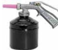
The Port-A-Blast sand blast gun is a complete sand blast unit. Fill the container with the abrasive material, connect the gun to your air line and it is ready to go to work. Will operate on air pressure as low as 60 PSI. However, for best results, pressures of 100-500 PSI are recommended. The greater the pressure the faster the cutting. The gun can be used to siphon abrasives or liquids
