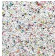
Removes paint/corrosion/rust from military, commercial and private aircraft while preserving anodized and alclad surfaces. Customers and usages include: Bell Helicopter Textron, U.S. Air Force, U.S. Navy, U.S. Marine Corps, U.S. Army, Pratt & Whitney, Commercial Airlines(MRO), FAA Repair Stations, turbine blades. **Note: Priced and sold in 25 lb bags.**
