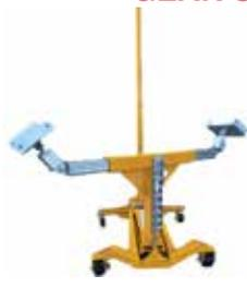
This simple, safe, and efficient design allows for quick servicing or repair of aircraft wheel assemblies and main gear security. The cushioned Belly Pad lifting option allows aircraft to be lifted from below the gearbox bulkheads. Lifting the aircraft from below allows the mechanic to inspect the security of the upper gear at the gearbox and to investigate any play or movement.
