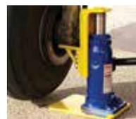
Aid aircraft maintenance, such as servicing brakes, working on bearings, or changing tires. Maximum load of 2,500 pounds and can be used on Piper aircraft, Musketeer, Mooney, and many more aircraft with near-vertical landing gear. Lower clearance lifting pad which allows jack owners to begin lifting from a 2 1/2" starting position and up to 12". It can be used on main gear, nose gear and the tail wheel. Made in USA.
