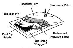
**VACUUM VALVE - TWO PIECE -** #8112 is a two-piece vacuum valve which requires one quarter turn to lock in place. Service temperature to 500° F. This valve is an industry standard The base is anodized and is red in color. Inside Diameter: 1/4" standard. Threads: 1/4" NPT.
