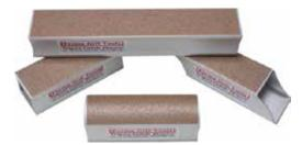
These user friendly sanding blocks are made from extruded, anodized aluminum. The 32mm (1.25") Radius Curve is covered on the external and internal radius with Tungsten Carbide abrasive sheets. The Contour Blocks come in either the Coarse (60US grit approx.) or Fine (120US grit approx.) Small block is 5.5" long and large block is 11" long. Benefits:
