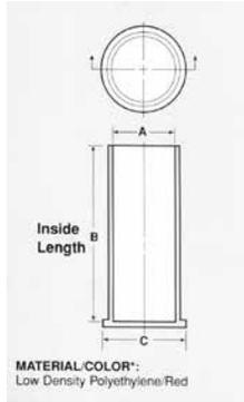
Series RCL caps are ideal for protecting threaded or smooth cylindrical surfaces. Originally designed for use on hydraulic double threaded bulkhead fittings, they are especially suitable where greater longitudinal protection is required.
