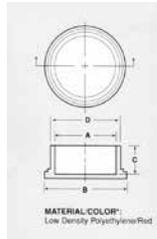
Static dissipative EC Series Capplugs provide positive ESD and physical protection for all common sizes of threaded electrical and electronic connectors. Also suitable for protecting non-threaded bayonet-type connectors.
