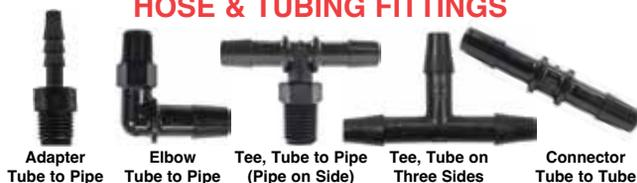
Hose and tubing Insert Fittings are available in high density black polyethylene or white Nylon. Use polyethylene fittings with Tygon, nylon or soft rubber tubing to assemble low pressure instrument lines such as airspeed pitot and static lines. Use Nylon fittings in gravity-feed fuel lines and engine breather lines.
