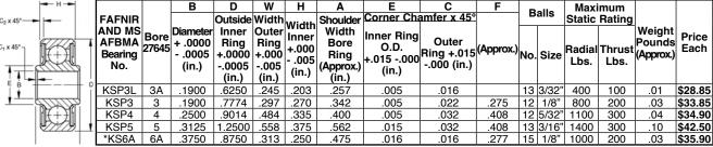
\* NOTE: These bearings are self-aligning for 10° in either direction except for KS6A (not AN200) which is self-aligning for 8° in either direction.
