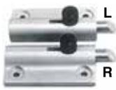
These universal spring loaded latches are designed for aircraft canopies, cockpit doors, and baggage doors. They are available in right hand and left hand models with different striker angle lock pins on the two models. These latches work great on a wide variety of experimental aircraft. Latch flange has 3/16" holes drilled for mounting.
