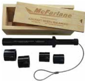
The Aircraft Wheel Balancer uses the same static balancing method that is used to balance helicopter rotors. The patent pending design features a pivot point that is easily adjustable on-the-fly for maximum sensitivity, and includes bushings to accommodate both 1 1/4" and 1 1/2" axle sizes.
