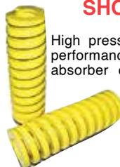
High pressure springs fabricated from alloy steel for top performance and long spring life. The Claude Gray shock absorber design has been service-proven on the EAA Biplane, Miniplane, Pitts and others. Over 1,000 pair in use. Length 6", 2" O.D., 1" I.D.. Wt. 4-1/2 lbs. per pair. Spring deflection 0.7" per 1,000 lb. force.
